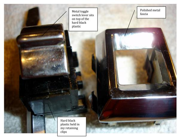
Once the center switch is separated from the polished metal fascia, lay the metal fascia upside down as depicted in the following picture. Note the position of the metal band clamps for reassembly. The metal band clamps are what holds the assembled switch in the door panel. They may be rusted and brittle so be careful
